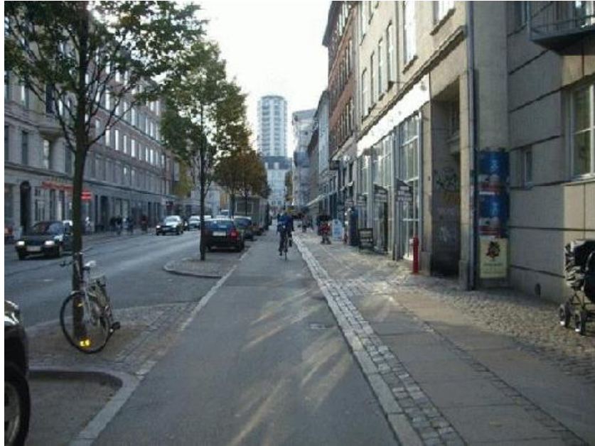
Figure 3—A Cycle Track in Copenhagen. Cycle tracks dramatically improve a bicyclist’s sense of safety by physically separating him or her from automobile traffic.
